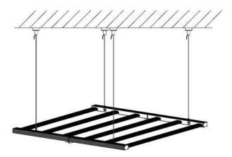
1. Hanging the lamp on the ceiling or other secure places with lifting rope.
