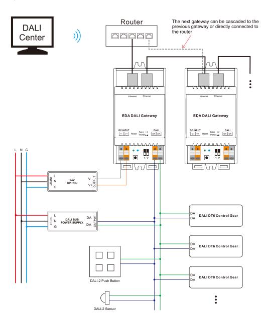
Note: When built-in DALI Bus PS is disabled, the number of following control gears depends on external DALI PS.
