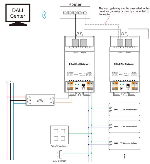
Note: Recommended no more than 8 sensors be installed on a single DALI bus.
