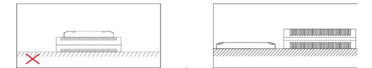
Direct contact between the load and the driver is prohibited when using the driver. Keep a certain distance between the driver and the load to avoid affecting the heat dissipation and lifetime of the drivers.
