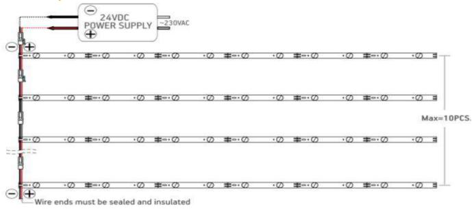
! 10PCS-max number of LED bars in one chain when the supplied from signle end. String end voltage can't be less thaan 23V,do not exceed specifie bar string length.
