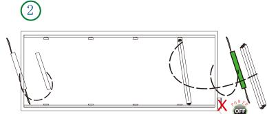
Step Two: remove all of the HO Lamps and Ballasts and dispose of them in accordance to local regulations. Do NOT disconnect existing wires from the lampholder terminals as you will need them again in step four.
