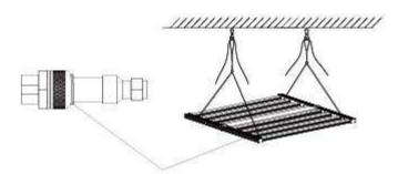
2. Connecting the wires from driver to the lamp, Note: the connector male plug arrow is aligned with the female plug arrow
