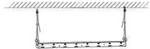
3. Install the lifting rope on the bracket first, then lock the lifting rope to the ceiling.
