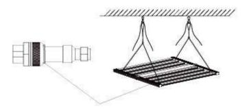
Connecting the wires from driver to the lamp, Note: the connector male plug arrow is aligned with the female plug arrow
