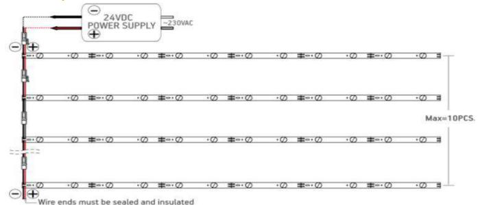
! 10PCS-max number of LED bars in one chain when the supplied from signle end. String end voltage can't be less thaan 23V,do not exceed specifie bar string length.
