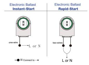
Step Four: re-wire the HOF lampholders. Ensure all lamps are oriented
