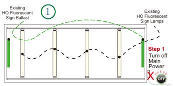
**Step One**: turn off main power to the sign or sign's branch circuit. In the event that there is no Disconnect Switch one should be added to meet code. Ensure proper grounding is bonded to the sign enclosure.
