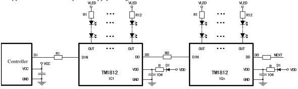
Resistance values of R1-R12 can be automatically adjusted based on the number of the LEDs cascaded at the OUT port, it is recommended to connect 100-200 Ohm resistor to RI and RO for signal isolation to prevent the effect of the lower level chip to the higher level chip.
