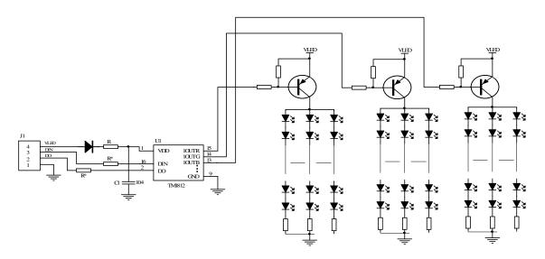
TITAN MICRO<sup>™</sup> 12-Channel Special Circuit for LED Driver Control TM1812 ELECTRONICS Packaging illustration SOP16
