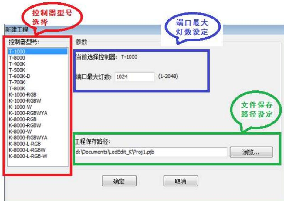
Note 1. Controller model selection: online controller model / offline controller model + lamp channel; where the lamp channel: RGB three channel / RGBW four channel / W single channel / RGBWYA multi channel.
