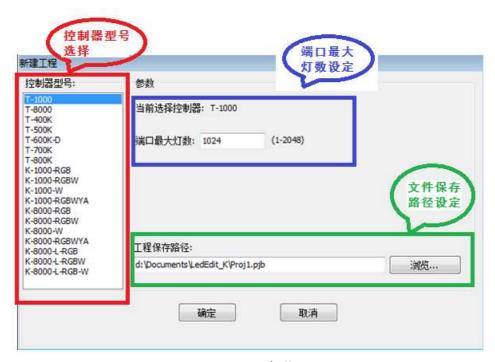
Note 1. Controller model selection: online controller model / offline controller model + lamp channel; where the lamp channel: RGB three channel / RGBW four channel / W single channel / RGBWYA multi channel.
