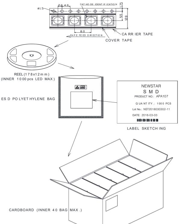
The reel pack is applied in SMD LED. The LEDs are packed in cardboard boxes after packaging in normal or antielectrostatic bags. cardboard boxes will be used to protect the LEDs from mechanical shocks during transportation. The boxes are not water resistant and therefore must be kept away from water and moisture.
