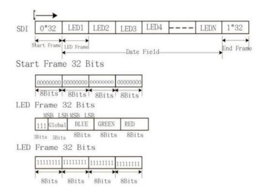
Global bit:5 bit (32 level) brightness setting, while controlling R,G,B three-color constant current output value, if set the global bit for the 10000( 16/31 ) is the output current is half again the original PWM settings
