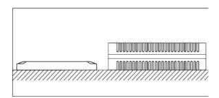
Direct contact between the load and the driver is prohibited when using the driver. Keep a certain distance between the driver and the load to avoid affecting the heat dissipation and lifetime of the drivers.
