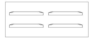
Do NOT stack drivers. Keep at least a certain distance between drivers when using them to avoid affecting the heat dissipation and lifetime of the drivers.
