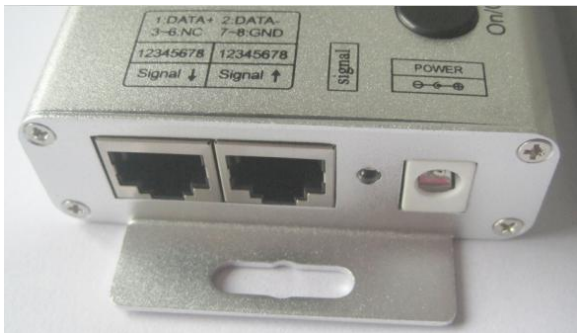
Power input: Adopt DC plug seat connector
